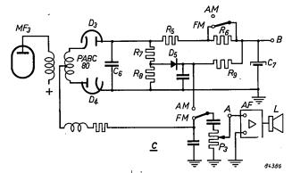
Fig. 12. a) Circuit of the ratio detector for FM. b) Circuit a modified to form an AM detector. c) Combination of both circuits, with two single-pole switches FM-AM.
