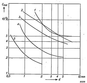
Fig. 3. Example of contrast-detail diagrams obtained by experiment. Object: 8 cm "Philite" + scatter grid.
