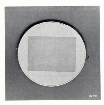
Fig. 7. The target of the "Scenioscope" is a thin plate of slightly conductive glass, from 50 to 70  $\mu$  thick, on a metal ring. The size of the rectangular area scanned is  $45 \times 60$  mm. The signal plate is a layer of metal on the back of the target.
