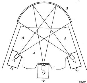
Fig. 1. Schematic diagram of the Cinerama system, showing the arrangement of the screen S, the three projectors  $P_1$ ,  $P_2$  and  $P_3$  in their projection rooms  $C_1$ ,  $C_2$  and  $C_3$ , and the audience A.
