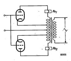
Fig. 9. Combination of two phase detectors, for use with a floating control with constant motor speed.
