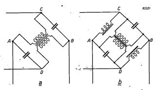
Fig. 4. The indeterminacy of the four arm currents in the Boucherot bridge can be eliminated by fitting the two coils on one core (a), or by coupling the capacitors across a 1:1 transformer (b).
