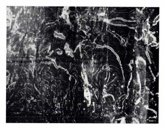
Fig. 9. Section of aluminium. An aluminium rod was shaped so that a small pyramid (about 0.3 mm high, base  $0.3 \times 0.3$  mm) stuck out at one end. The tip of this was cut with a diamond knife. The angle between knife and specimen was very critical; the best adjustment was found empirically. No further particulars can yet be given about the structure seen in the photograph. Magnification  $24\,000\,\times$ .
