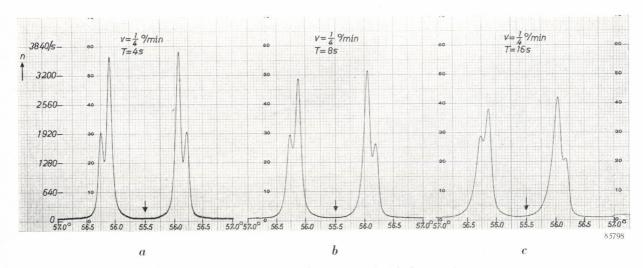
Fig. 6. a-c) The same diffraction line as in fig. 5, recorded with the counting-rate meter at a scanning speed  $v=\frac{1}{4}^{\circ}$  per min and three values of the time constant T. All other conditions same as in fig. 5. Note that the deterioration of line shape with increasing T is similar to that in fig. 5. The number of counts in corresponding angular intervals, however, is the same for all three recordings.
