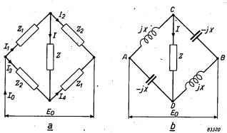
Fig. 3. a) Bridge circuit with two impedances  $Z_1$  and two impedances  $Z_2$  in the arms, and a load impedance Z in one of the diagonals.
