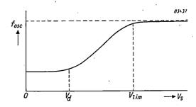
Fig. 6. The frequency  $f_{\rm osc}$  of the oscillator (13 in fig. 4) as a function of the signal voltage Vs. The threshold voltage is  $V_{\rm d}$ , the limiting voltage  $V_{\rm lim}$ .
