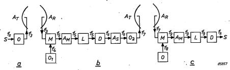
Fig. 2. Block diagrams of a transmitter (a), a relay station (b), and a terminal station (c), using an oscillating transmitting tube and a system of single modulation. The significance of the letters is given in the text.
