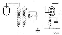
Fig. 5. Coupling between two stages of the vision I.F. amplifier. 1 primary, 2 secondary coil of the coupling transformer. 3 filter tuned to the frequency of an interfering signal.
