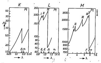
Fig. 9. Mass absorption coefficient  $(\mu/\varrho)$  of platinum as a function of wavelength  $\lambda$  in the regions of the K, L and M absorption edges. Some characteristic emission lines of the K, L and M series of platinum are shown with arrows.
