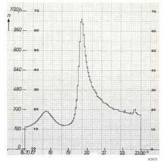
Fig. 14. Part of recording of a diffraction pattern  $(16.7^{\circ} < 2\Theta < 23.0^{\circ})$  made with the counting rate computer. Montmorillonite (dry specimen), CuKa radiation with nickel filter, steps  $0.05^{\circ}$  with N=6400; recording time  $2\frac{3}{4}$  hours.
