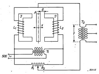
Fig. 7. Schematic diagram of inductive displacement pick-up. The coils  $L_1$  and  $L_2$ , together with the resistors  $R_1$  and  $R_2$ , form a bridge circuit fed by an valve oscillator (500 c/s) via transformer  $T_1$ . The bridge is balanced if armature A is located mid-way between the yokes J. If the armature is located to the left or to the right of the centre, a voltage  $\gamma$  is produced across the primary of the output transformer  $T_2$ .
