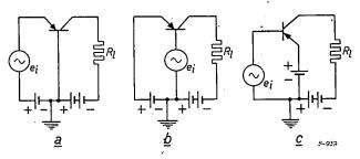
Fig. 7. a) Transistor circuit with common base. If the internal resistances of the D.C. sources are neglected, then A.C. input source  $e_i$  and load resistance  $R_l$  are both connected directly to the base lead of the transistor.
