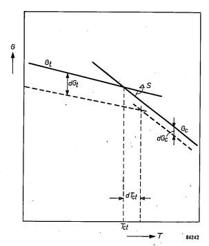
Fig. 2. Variation of the Gibbs free energy G with the temperature T (schematic) for cubic  $BaTiO_3$  ( $G_c$ ) and for tetragonal  $BaTiO_3$  ( $G_t$ ). The point of intersection of these lines gives the transition temperature  $T_{ct}$ . This point is displaced if, for any reason, the lines  $G_c$  and  $G_t$  are moved over different distances  $dG_c$  and  $dG_t$ .
