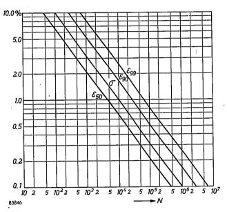
Fig. 3. Probable fractional error  $\varepsilon_{50}$  of counting rate, and 90% and 99% confidence limits  $\varepsilon_{90}$  and  $\varepsilon_{99}$ , as functions of the accumulated number of counts N, for a Gaussian distribution.
