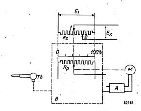
Fig. 2. Use of the automatic potentiometer for control of the temperature of a furnace. B measuring circuit; Th thermoelement;  $R_p$  measuring slidewire; A amplifier; M drive motor;  $R_z$  control slidewire. The contact I is mounted on the same carriage as the contact of the measuring slidewire. Contact I is set to a position corresponding to the desired temperature.
