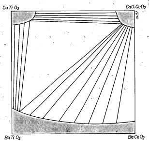
Fig. 10. Phase diagram for the system BaTiO<sub>3</sub>-CaTiO<sub>3</sub>-CaO. CeO<sub>2</sub>-BaCeO<sub>3</sub> (schematic). In this diagram, besides the two perovskite phases, a third phase with fluorite structure, occurs in the CaO.CeO<sub>2</sub> corner. The Gibbs free energy is so small there that the disposition of the connodes in this diagram differs from that in fig. 7.
