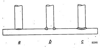
Fig. 1. Difference between the welds produced by the various methods of stud welding.
