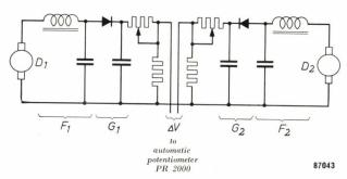
Fig. 5. Circuit diagram of the "Knijp van Jut" (Test your Clench).  $D_1$ ,  $D_2$  are hand-dynamos;  $F_1$ ,  $F_2$  low-pass filters and  $G_1$ ,  $G_2$  rectifiers.
