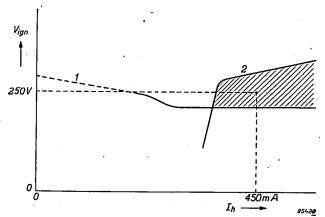
Fig. 3. Curve  $I: V_{\text{ign}}$  as a function of  $I_h$  for the lowest ambient temperature at which the lamp must still ignite, modified by a safety factor which takes into account the spread between lamps and mains voltage fluctuations.
