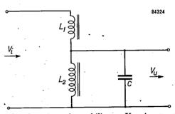
Fig. 3. Simple magnetic stabilizer.  $V_{\rm i}=$  input voltage.  $V_{\rm u}=$  output voltage,  $L_{\rm 1}=$  non-saturated choke,  $L_{\rm 2}=$  saturated choke. The resonant circuit  $L_{\rm 2}C$  is in resonance at one particular voltage.
