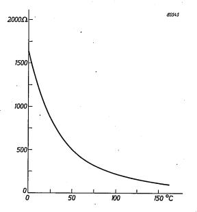
Fig. 4. The resistance of an NTC resistor as a function of the temperature.
