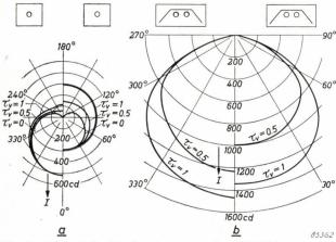
Fig. 6. a) The light distribution curves for "TL"F lamps with dirt layers on the upper half having the same values of  $\tau_{\rm V}$  as in fig. 2a are shown on the left. The slot is directed downwards. For comparison purposes, the curves of fig. 2a for the normal lamp are reproduced on the right.
