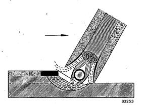
Fig. 2. A deep "cup", formed at the tip of a contact welding electrode during the deposition of metal, prevents the electrode from "freezing" to the work.
