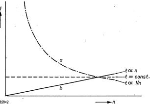
Fig. 11. The relative statistical error  $\varepsilon$  and required counting time t, as functions of the counting rate n, for three different types of counting strategy.
