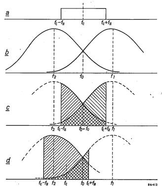
Fig. 1. a) The transmitted frequency band, showing the central frequency  $f_c$  and frequency swing  $f_z$ . The signal strength is plotted vertically.
