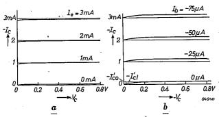
Fig. 9. Theoretical characteristics of a transistor: collector current  $I_c$  as function of the collector voltage  $V_c$  for various values of the input current. According to the sign convention (fig. 4)  $V_c$  and  $I_c$  are negative:  $-V_c$  and  $-I_c$  have therefore been plotted.
