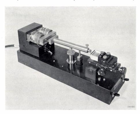
Fig. 1. The new ultramicrotome designed at Eindhoven.
