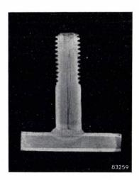
Fig. 12. Cross-section of a  $\frac{1}{2}$ -inch stud welded to a plate by the cartridge method of stud welding. The slag enclosures revealed by etching show that the stud and the plate are both made of rimmed steel <sup>4</sup>).
