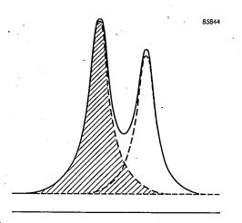
Fig. 17. The area of slightly overlapping diffraction lines reflected from different lattice planes can be integrated by sketching in the "tails" of the lines in the overlapping region and using a planimeter.
