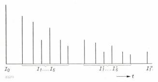
Fig. 4. If a report (pulse  $I_0$ ) is produced in a hall with stereo reverberation, the six loudspeakers deliver during one revolution of the delay wheel the six reports  $I_1...I_6$ . If electrical feedback is applied from the sixth play-back head to the recording head, the loudspeakers give a second series of six reports  $(I_1...I_6')$ , a third, and so on. (Acoustic feedback is here neglected.)
