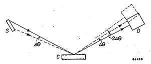
Fig. 14. When the parallel slit system is omitted, the analyzing crystal when being rotated will continue to contribute rays reflected at a given angle  $\Theta$ , within a certain angular region  $\Delta\Theta$  determined by the size of the specimen. The region is limited by the introduction of the parallel slit system.
