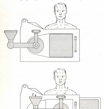
Fig. 9. Top: The apparatus as used with an ordinary fluorescent screen. Bottom: With the image intensifier positioned in front of the patient. For the meaning of the letters see fig. 2 and fig. 8.
