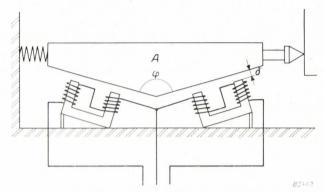
Fig. 10. Displacement pick-up for measuring the absolute change in length of the casing. The principle is the same as that of the pick-up of fig. 7, but owing to the tapered shape of armature A, a change in length of the shaft now corresponds to a 50 times smaller change of the air gap  $\delta$ . The angle  $\varphi$ , actually about 178°, is shown smaller for the sake of clarity.
