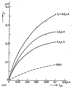
Fig. 12. Full curves:  $I_s$  as a function of  $I_{\rm ph}$  for the "Scenioscope" for various values of the leakage current  $I_l$  through the glass target ( $I_l$  measured in darkness). Broken curve:  $I_s = f(I_{\rm ph})$  for image iconoscope 5854 (from fig. 4).
