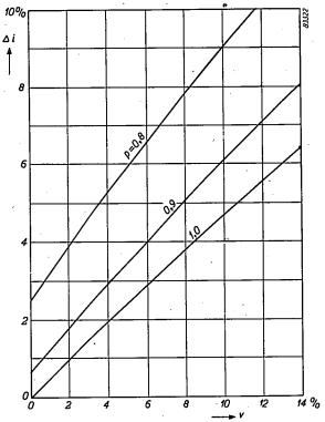
Fig. 5. The relative current difference  $\triangle i$  plotted against the relative loss v in the Boucherot bridge, for various values of the detuning p. Almost identical curves hold good for the reciprocal values of p.
