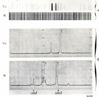
Fig. 1. a) Optical spectra of copper and tungsten in the region 3000 to 3500 angstroms. b) X-ray spectra of same elements.
