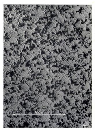
Fig. 2. Photomicrograph showing a polished section of the tungsten surface after the volatilization of the copper. The average pore size is of the order of a few microns, the pore separation varying between a few microns and a few tens of microns. (Such small pore distances are desirable for the surface of dispenser cathodes <sup>7</sup>).)
