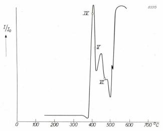
Fig. 7. Recorded gloss curve of an experimental glaze prepared in the laboratory. The heating-rate was 2 °C per minute. As the heating-rate increased, the curve was displaced as a whole towards somewhat higher temperatures without appreciable changes in the various features of the curve.
