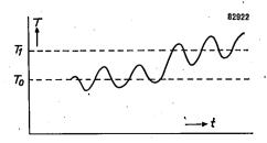
Fig. 6. The temperature T of a furnace as a function of the time t for a system of three-step control, the external conditions being such that the furnace temperature has a tendency to rise continuously.
