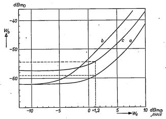
Fig. 13. a) Experimental curve, showing the noise power  $W_b$  in one of the 8 free channels as a function of the power  $W_s$  supplied to the remaining 40 channels.
