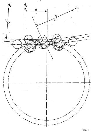
Fig. 8. The teeth of one of the rotating sprocket wheels and the rollers of the sprocket engaging with it (rotation about axis  $A_1$ ), in three consecutive positions. Instead of being vertically below axis  $A_2$ , the sprocket wheel axis is displaced a certain distance ( $\Delta$ ) inwards.
