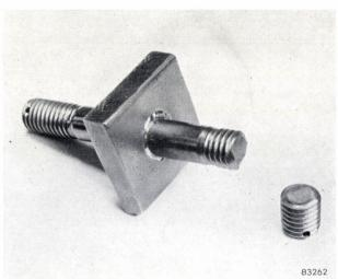
Fig. 14. a) Result of a tensile test on two studs welded end to end to oposite sides of a plate.
