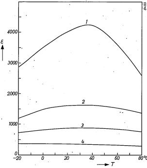
Fig. 8. ε-T curves for sintered specimens prepared from BaCO<sub>3</sub>, CaCO<sub>3</sub>, TiO<sub>2</sub> and ZrO<sub>2</sub>, corresponding to the compositions 1 to 4 in fig. 7. Here too, the strong flattening action of the increasing proportions of the phase rich in CaTiO<sub>3</sub> is demonstrated.
