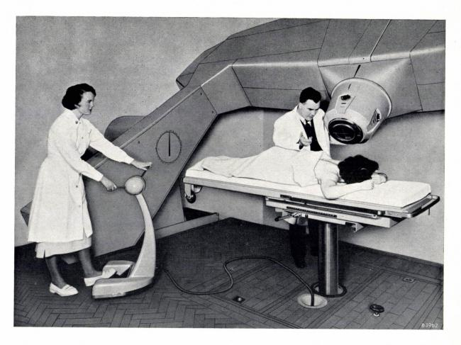
Fig. 1. Medical linear accelerator generating 4 MeV X-rays, installed at Newcastle Genera Hospital (England). This was the first of a series of 4 MeV-accelerators to be used for deep X-ray therapy.
