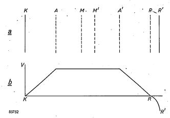
Fig. 1. a) Diagram showing the principle of the multi-reflex klystron. K cathode; A and A' grids forming the anode; M and M' grids of the modulator system; R and R' repeller electrodes.
