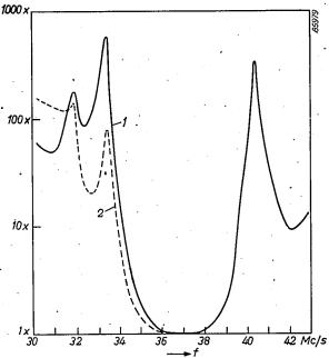
Fig. 6. Selectivity characteristic of the vision I.F. amplifier  $(MF_1$  in fig. 7), I for the Belgian standards and the Gerber standard, 2 for the French standard.
