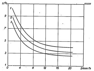
Fig. 3. Wire-sensitivity (in % of thickness of object) in the fluoroscopy of steel with an X-ray image intensifier, plotted against the thickness of the material (in mm). Tube voltage 80 to 150 kV, distance between focus and intensifier 50 cm, size of focus  $0.4 \times 0.4$  mm. Enlarged X-ray shadow picture projection: the magnifications associated with curves 1, 2 and 3 are 1.2, 1.6 and 2.2, respectively.
