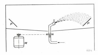
Fig. 5. The apparatus in fig. 4 is seen from above and in section. The sprayer S is rotated about a vertical axis by an electric motor M, and plays successively on the glass slides P which have been treated with the preparations whose sticking power is to be investigated. A rainfall of 1 cm per hour is employed for a period of 1 to 2 hours.
