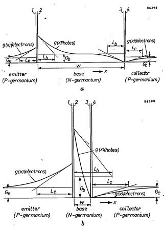
Fig. 6. Minority concentrations g(x) in the emitter and in the collector (electrons) and in the base (holes) of a P-N-P transistor, as functions of position x.
