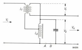
Fig. 4. Stabilizer similar to that of fig. 3, with compensation winding on  $L_1$ . Here  $L_2$  is in the form of an autotransformer, so that  $V_{\rm u}$  is equal to the nominal value of  $V_{\rm i}$ .
