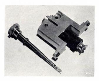
Fig. 15. The specimen stage and specimen holder (left). The cylindrical central section of the specimen stage contains a vacuum lock through which the specimen holder is inserted into the microscope tube.
