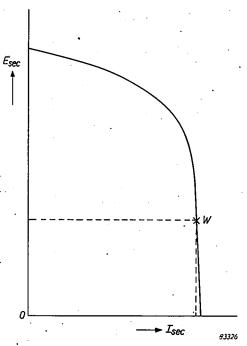
Fig. 12. The secondary voltage  $(E_{\rm sec})$  plotted against the secondary current  $(I_{\rm sec})$  of a lamp transformer loaded with a variable resistor. The primary winding of this transformer is included in a series circuit supplied by a Boucherot bridge. The curve should be steep at the working point W, and the voltage at  $I_{\rm sec}=0$  should not be unduly high.
