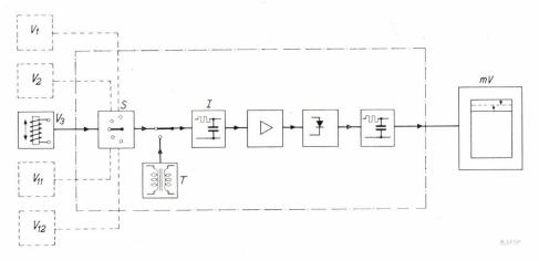
Fig. 5. Block diagram showing the connection of the vibration pick-ups  $V_1...V_{12}$  (7 in fig. 1) alternately connected via a rotary switch S to the integrating network I. The output voltage of I is applied via an amplifier, a rectifier and a smoothing filter to a recording millivoltmeter mV (see fig. 6). T calibration transformer.
