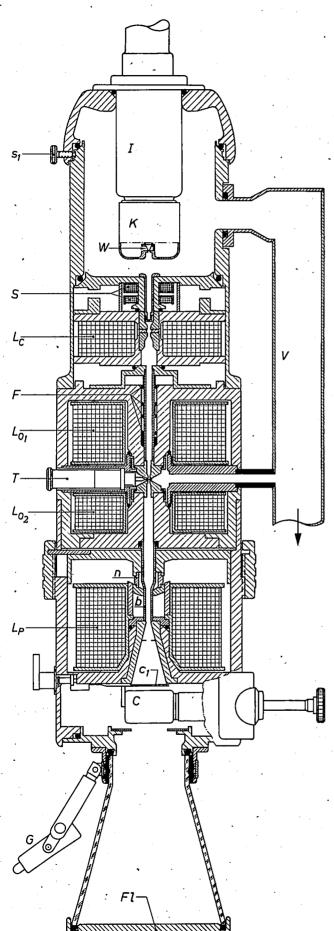
controls the focal length, and with it the angular aperture, of the beam falling on the specimen so as to give the image on the fluorescent screen the required degree of brightness. The lens, together with the electron gun, is mounted in a tube which can be moved bodily in a transverse direction (the adjusting screws for this purpose have not been drawn). In this way the electron gun and condensor lens combination can be accurately centred with the objective lens.
