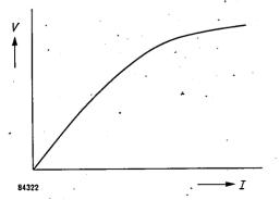
Fig. 1. Relationship between r.m.s. current and voltage for a choke with soft-iron core.
