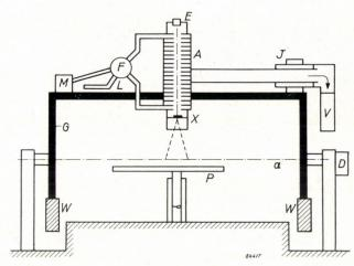
Fig. 2. Schematic representation of the machine shown in fig. 1. A is the accelerator proper (corrugated waveguide 1 metre long), mounted in gantry G rotatable about the axis a by means of an oil motor D. E electron gun, X X-ray head, M magnetron, F feedback bridge, V diffusion pump, J rotating vacuum joint, W counterweights, P patient's couch, L water load.
