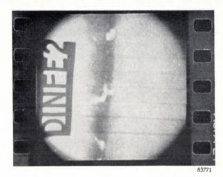
Fig. 5. Welded seam in steel sheet 15 mm thick, photographed with the image intensifier. Note the faultsin the seam, and the shadow of the DIN test-object placed in front of the plate. X-ray tube data: 140 kV, 3 mA; focus  $0.4\times0.4$  mm. Exposure 15 seconds.
