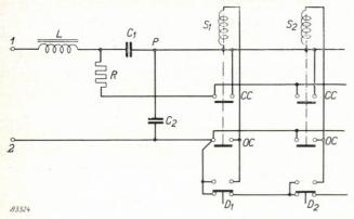
Fig. 7. Interlock mechanism to preclude the possibility that two or more switches (with energising coils  $S_1, S_2, \ldots$ ) will be closed at the same time. I, 2 terminals of the mains supplying the control voltage; L- $C_1$  resonant circuit; R damping resistor; CC short-circuit contacts of  $C_1$ ; OC transfer contacts  $C_2$  auxiliary capacitor;  $D_1, D_2, \ldots$  push buttons.
