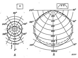
Fig. 3. Light distribution curve of the new 40 W "TL"F lamp with directional radiating characteristics (a) and for two of these lamps in a trough fitting (b). For comparison purposes the corresponding curves for the normal lamp, taken from fig. 1a and b, are indicated with broken lines.
