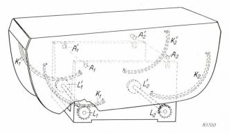
Fig. 6. Schematic drawing of the driving mechanism of the table. The table carries two heavy sprockets acting as toothed segments,  $K_1-K_1{'}$  and  $K_2-K_2{'}$ , centring upon the two axes of rotation,  $A_1-A_1{'}$  and  $A_2-A_2{'}$ , respectively, These sprockets engage with two pairs of sprocket wheels,  $L_1-L_1{'}$  and  $L_2-L_2{'}$ , which are driven (at the same speed and in the same direction) by a centrally mounted motor (see fig. 9).
