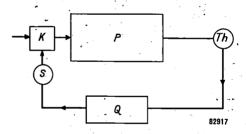
Fig. 1. Diagram of a closed loop automatic control system. The process to be controlled is represented by P. The measuring element; Q controller; S motor element; K correcting element.
