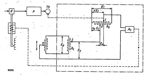
Fig. 14. Diagram of a circuit for control by time-proportional switching. The contact 4 is moved up and down periodically at a constant rate.
