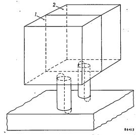
Fig. 2. The two cavity resonators l and 2 are symmetrically coupled to the wave guide in a plane perpendicular to the direction of propagation.
