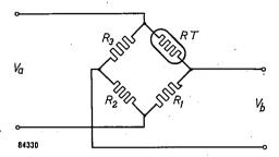
Fig. 11. Detecting device of the "Balham" stabilizer.  $V_a$  is proportional to the output voltage of the stabilizer. RT is a thermistor; its resistance is strongly dependent upon the temperature. At the normal value of  $V_a$  the bridge is just balanced. If  $V_a$  assumes a higher or lower value, the temperature of RT will change, so that the bridge becomes unbalanced. This causes a relationship similar to that of fig. 8 between  $V_a$  and  $V_b$ .
