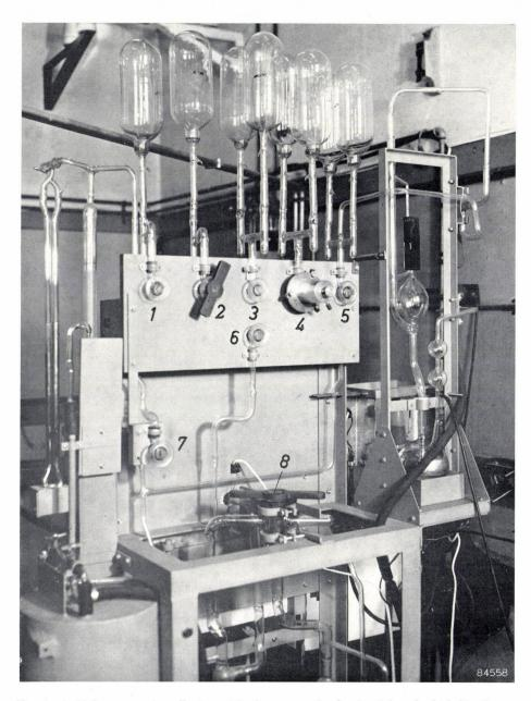
Fig. 3. A high-vacuum installation with nine taps as in fig. 2, eight of which  $(l - \theta)$  may be seen. A cap is attached to tap 4, and operating keys to 2 and  $\theta$ .
