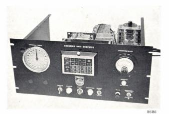
Fig. 1. Chassis and front panel of the "Norelco" counting-rate computer. This unit is placed in the electronic circuits rack of the diffractometer. The computer output can either be fed to the recorder or be read on the meter at the upper right. At the upper left a register is mounted which is not used for the computer but only in manual fixed count measurements (cf. II).
