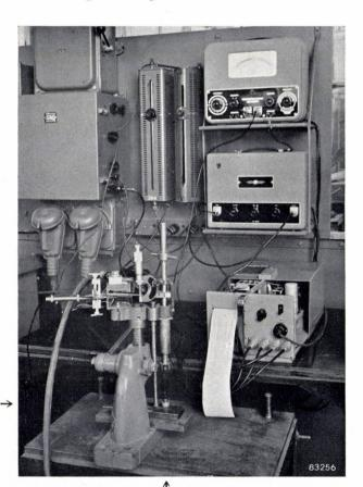
Fig. 11. The equipment employed to record variations in the voltage and the current, and in the distance between the stud and the work, as a function of time during the welding process. The ordinary welding gun was not employed during these measurements. The arrows indicate the position of the welding cartridge.
