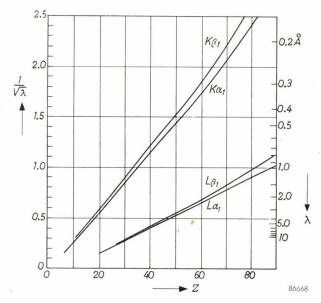
Fig. 3. Wavelengths  $\lambda$  of characteristic X-ray spectral lines of elements, plotted against atomic number Z. According to Moseley's law, there should be a linear relationship between  $1/|\overline{\lambda}|$  and Z.
