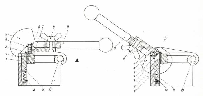
Fig. 2. Structural design: I clamping piece; 2 support bar; 3 radius plate; 4 test specimen; 5 cam, which depresses support bar; 6 rollers, mounted in thrust block 7, which is fixed by wing-nut 8 to lever 9; the excentric 10 serves to hold clamping piece against specimen; 11 pin by which the support bar is depressed against spring 12. a) Machine ready for operation after insertion of test specimen; b) after bending through  $145^{\circ}$ .
