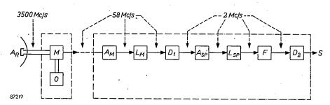
Fig. 10. Block diagram of the receiver of fig. 9. The left-hand section (surrounded by dotted line) is built into the reflector assembly; the right-hand part is incorporated in the rack.
