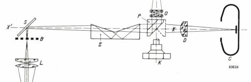
Fig. 2. Schematic cross section of the optical system. The objective O forms an image B of the viewing screen A of the image intensifier tube, via the roof prism P, erecting prism Z and mirror S. Image B is observed through a magnifying eyepiece L. Section S-L rotates about axis X-X', thus enabling L to be adjusted to eye-level. Knob K turns prism P.
