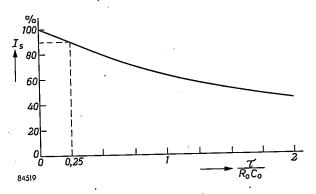
Fig. 9. Signal current ( $I_s$ ; on relative scale), plotted as a function of  $\tau/R_0C_0$ . The values of  $R_0$  and  $C_0$  are chosen so as to give an  $I_s$  equal to 90% of the maximum value ( $\tau/R_0C_0=0.25$ )
