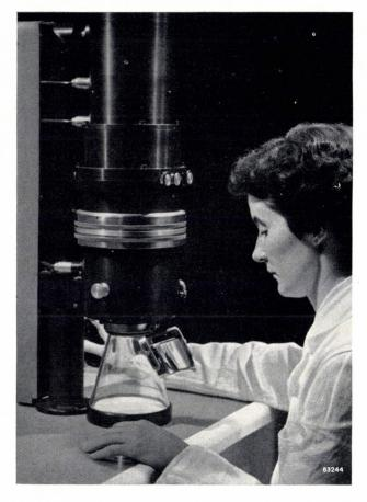
Fig. 13. The microscope tube of the EM 75 kV. By turning the milled ring which encloses the tube, the upper pole piece of the projector lens is displaced. The ring can make  $^{7}/_{8}$  of a complete turn; this causes the pole piece to move 15 mm in a vertical direction, which alters the magnification by a factor 9. The wall of the vacuum tube is here formed by a thin brass tube (b in fig. 12), which makes a sliding fit in theb ore of the pole pieces, which are thus outside the vacuum.
