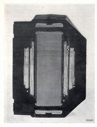
Fig. 16. Cross-section of the rubber-cased transformer shown in fig. 15. It will be seen that the turns are completely enclosed in rubber, which has penetrated into the spaces between them.
