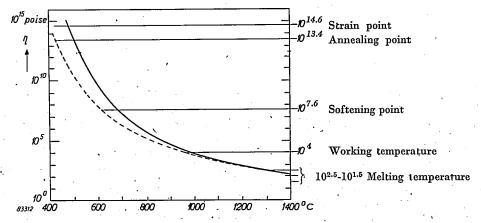
Fig. 1. The viscosity  $\eta$  (in poise) of two types of glass as a function of the temperature. The full curve applies to soda glass, the dashed curve to lead glass. For processing, certain values of  $\eta$  are required, which thus determine the processing temperatures.
