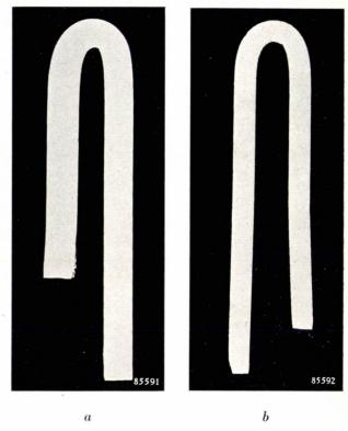
Fig. 3. a) Section of a test specimen of chrome steel, bent through  $180^{\circ}$  by the machine shown in fig. 1 (tensile strength of specimen approx. 65 kg/mm²; specimen thickness d=1.9 mm; diameter of radius plate D=0.95 mm; thus D/d=0.5). b) Section of a test specimen of mild steel (tensile strength approx. 40 kg/mm²; d=1.0 mm; D=1.2 mm, and D/d=1.2).
