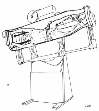
from the patient, a movement which needs no balancing against the force of gravity. Moreover, apparatus so designed eliminates the above-mentioned problems associated with the interchanging of the different attachments for viewing and recording the X-ray image. Also, the radiologist can be given
