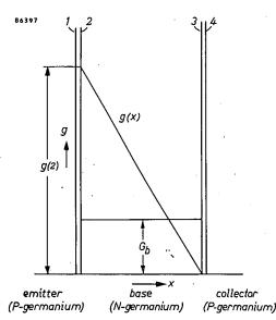
Fig. 5. To explain the essential principle of transistor action, the concentration of only the minority charge carriers g(x) in the base of a junction transistor is given as function of position x.  $G_b$  represents the equilibrium concentration of the minority charge carriers in the base.
