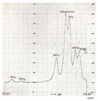
Fig. 2. Chart of diffraction pattern recorded by the "Norelco" counting-rate computer. The Bragg angle steps in this instance are  $0.02^{\circ}(2\Theta)$ ; the statistical error  $\varepsilon_{50}$  of each point is 0.8%. This recording took about 3 hours of completely automatic operation.
