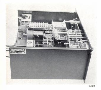
Fig. 4. Computer chassis. A number of elements shown in fig. 3 are visible; the lettering is identical to that of fig. 3. To the extreme left is a multiple-deck motor-driven cam switch S which controls each cycle of the operation of the computer.
