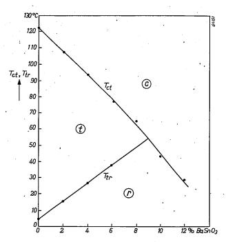
Fig. 4. The effect of  $BaSnO_3$  on the transition points of  $BaTiO_3$  (an almost similar figure applies for additions of  $BaZrO_3$ ) c = region of cubic structure, <math>t = tetragonal, r = rhombic.
