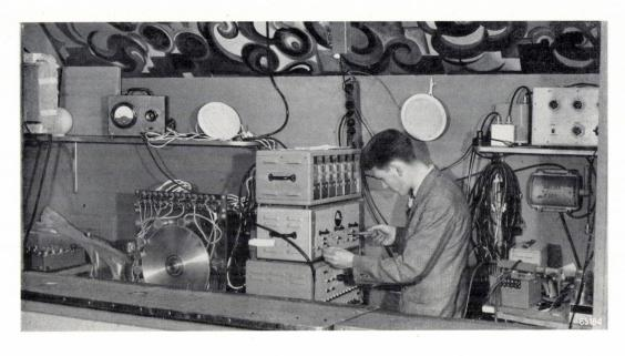
Fig. 3. Stereo reverberation installation in the "Gebouw voor Kunsten en Wetenschappen" (Arts and Sciences Hall), The Hague, in experimental form. The delay wheel was then fitted with ten play-back heads, of which six could operate simultaneously. It was possible to switch over rapidly from one set of play-back heads to another.
