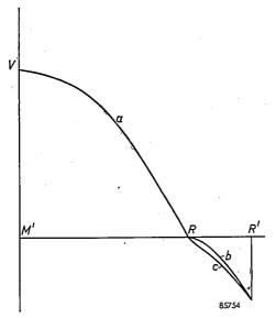
Fig. 3. The static potential between the planes M' and R' of fig. 1. a) the ideal potential between M' and R: a parabolic curve. b) and c) The potential slopes between R and R' corresponding to the transit time curves  $\tau_2$  and  $\tau_3$  respectively.
