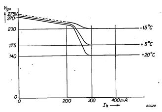
Fig. 2. Relation of ignition voltage  $V_{\rm ign}$  of the "TL"M 40 W lamp to the electrode heating current  $I_{\rm h}$ , for various ambient temperatures.
