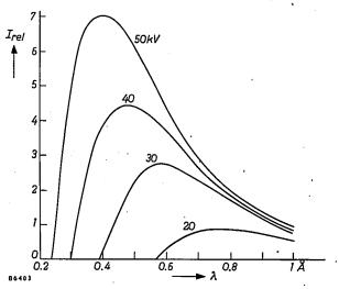
Fig. 8. The continuous spectrum of a tungsten target X-ray tube (relative intensity  $I_{\rm rel}$  vs. wavelength  $\lambda$ ) obtained with various voltages (peak values) and the same tube current. The curves were redrawn from separate rate meter recordings. Experimental conditions: full-wave rectification, silicon crystal analyzer (111-plane), scintillation counter.
