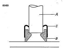
Fig. 4. The welding cartridge, comprising a semi-conductive igniter element B and a cardboard collar C to hold it on the stud to be welded A. During welding, the ridge of the igniter element supporting the stud melts, thus enabling the stud to be pressed into the pool of molten metal.
