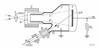
Fig. 2. Schematic cross-section of the image iconoscope. L lens; P photo-cachode; S coil of the magnetic electron lens; T target (mica); C collector; E scanning beam supplied by an electron gun of which only the cathode K is shown in the diagram; F focusing coil; D deflecting coils; SP signal plate;  $R_s$  signal resistor.
