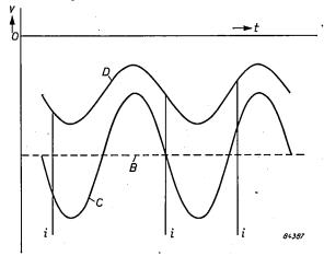
Fig. 13. The straight line B and curves C and D give the voltage variations at the points B, C and D respectively in fig. 12b with respect to earth (0). Interference pulses are clipped at the level B.
