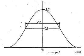
Fig. 5. Sinusoidal band-pass response of the I.F. filter.
