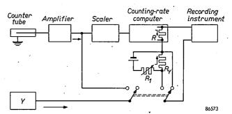
Fig. 7. Block diagram showing the provisions made for the application of the Cooke-Yarborough method to the computer. The pulse generator Y is connected to the input of the scaling circuits in parallel to the detector. At the same time a resistor R carrying a constant current (adjusted once and for all by means of a rheostat  $R_1$ ) is connected in series with the resistor R through which the output current of the computer is fed. The voltage across  $R+R_Y$  is fed to the recorder.
