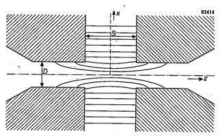
Fig. 6. The configuration of a magnetic lens is characterised by the diameter D of the bore through which the electrons pass (z-direction), and the width S of the gap between the pole pieces.
