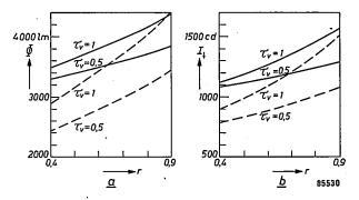
Fig. 10. a) Effect of the reflection factor r of the reflector of a two-lamp trough fitting on its luminous flux. The full lines refer to "TL"F lamps, the dotted lines to normal lamps. Both types of lamp were measured in a clean condition  $(\tau_{\rm v}=1)$  and with a layer of dirt on the upper surface  $(\tau_{\rm v}=0.5)$ . b) As for (a), but showing the effect on the luminous intensity vertically downwards,  $I_{\psi}$ .
