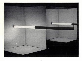
Fig. 5. a) "TL" lamps in operation; a normal lamp and a lamp with directional distribution ("TL"F lamp, in the foreground). In the "TL"F lamp the brightness is low where the reflecting layer is present between the fluorescent powder layer and the glass wall. The light is mainly emitted through the bright slot (angular width about 130°).
