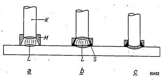
Fig. 3. The different stages in stud welding with a partially stripped contact welding electrode having a "cupped" tip. M portion of coating left on the rod, K core wire, L molten pool of metal, S slag.
