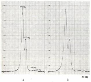
Fig. 10. Diffraction lines (quartz 1122 and 0003) recorded with the counting-rate meter: a) step scanning with  $0.02^{\circ}$  steps, counting time interval for each step 30 sec, time constant T=4 sec; b) continuous scanning at  $v=\frac{1}{8}^{\circ}$  per min.
