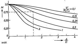
Fig. 10. Relative modulation depth M of the potential pattern on the target, plotted against  $\Delta/D$  ( $\Delta=$  thickness of target, D= width of bands in a picture comprising black and white bands), for various values of  $\tau/R_0C_0$ . With  $\tau/R_0C_0=0.25$ ,  $\Delta/D$  must not exceed roughly 1.5 if the modulation depth is to be maintained at a reasonable value.
