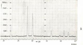
Fig. 9. Diffractometer pattern of  $Sr(NO_3)_2$  obtained with  $CuK\alpha$  radiation, 30 kV peak, 20 mA.
