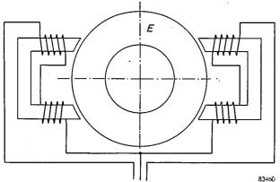
Fig. 12. Inductive displacement pick-up (cf. fig. 7) in a form suitable for measuring the eccentricity of the shaft. Here the armature consists of a disc E (of "Permenorm"), fitted on the shaft.
