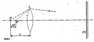
Fig. 3. If the acceleration voltage of the electrons or the excitation current of the objective L vary, the image on the fluorescent screen Fl is not that of the object plane P, but is the image of a plane P' displaced by  $\Delta v$  from the object (v) is the distance between object and objective lens).
