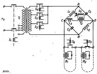
Fig. 6. Simplified circuit diagram of a low power supply unit.  $S_1$  main switch;  $T_1$  isolating transformer;  $S_2$ ,  $S_3$ ,  $S_4$  luminous intensity selectors (varying in number from 0 to 5); ABCD Boucherot bridge;  $L_3$  choke to limit the output voltage when the runway circuit is interrupted;  $T_2$  current transformer;  $S_5$  relay, which, when energised, opens mains switch  $S_1$ ;  $B_1$ ,  $B_2$  runway light circuits;  $S_6$ ,  $S_7$  runway selectors.
