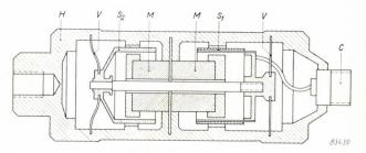
Fig. 2. Cross section of the electro-dynamic vibration pick-up PR 9260. M permanent magnet, mounted in the housing H.  $S_1$  output coil (with connection contact C).  $S_2$  damping coil (copper sleeve acting as a short-circuited winding). The coils are mechanically connected and suspended between the spring membranes V.
