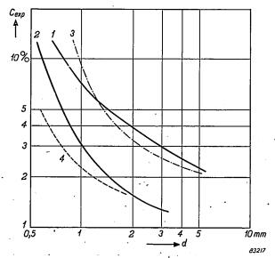
Fig. 4. Example of contrast-detail diagrams obtained by experiment, analogous to fig. 3. Object: 8 cm "Philite" + scatter grid.
