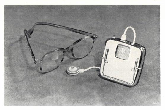
Fig. 1. The hearing-aid KL 5500 which works on transistors.
