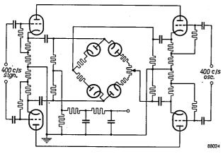
Fig. 4. Simplified circuit of the synchronous detector.
