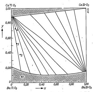
Fig. 7. Phase diagram at 1300 °C of the system BaTiO<sub>3</sub>-CaTiO<sub>3</sub>-GaZrO<sub>3</sub>-BaZrO<sub>3</sub> with two perovskite phases (shaded areas). The ratio Zr/Ti is x/(1-x), the ratio Ca/Ba is y/(1-y). The straight lines in the segregation region are the connodes. From the direction of the connodes it can be seen that the combination BaZrO<sub>3</sub> + CaTiO<sub>3</sub> is more stable than the combination BaTiO<sub>3</sub> + CaZrO<sub>3</sub>.
