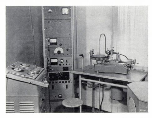
Fig. 1. Equipment for the transfer of magnetic recordings onto lacquer discs. From left to right: the machine in which the magnetic recording is played back, the amplifier rack (also containing other electronic apparatus), the machine on which the lacquer disc is engraved, and a monitoring loudspeaker.
