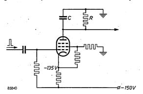
Fig. 4. Basic circuit of the counting-rate meter. The pulses arising in the counter tube are fed to the control grid of a pentode. Since the anode current of the pentode is nearly independent of the anode voltage, a constant charge is passed through the pentode for every pulse, independent of the charge already present on the capacitor C. The voltage produced across the resistor R is smoothed by C.
