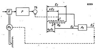
Fig. 8. Scheme for floating control. The motor  $M_1$  actuated by the output voltage  $E_{x'}$  of the amplifier  $A_1$ , changes the position of the correcting element K.
