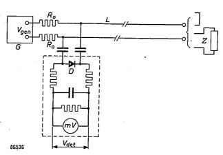
Fig. 9. Circuit for measuring impedances. G is a signal generator with adjustable frequency and voltage, amplitude-modulated. L is a long transmission line. Z is the impedance to be measured, D the detector and mV the electronic millivoltmeter.
