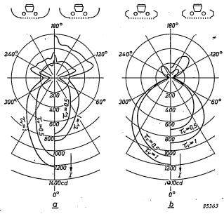
Fig. 11. a) Light distribution curves for a louvred fitting with translucent side-panels (see insets). The left-hand curves are for clean "TL"F lamps ( $\tau_{\rm v}=1$ ) in a clean fitting, and for dirty "TL"F lamps ( $\tau_{\rm v}=0.5$ ) in a correspondingly dirty fitting; the right hand curves are for normal "TL" lamps under the same conditions.
