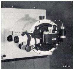
Fig. 5. Binocular microscope and camera, mounted so that they can be swung alternately into position in front of the image intensifier. The left-hand picture shows the microscope in use; in the right-hand picture the camera is in use.
