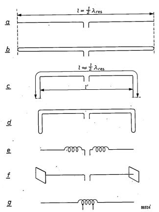
Fig. 7. Forms of dipole aerials. a) Normal dipole; length l equal to half the resonance wave length  $\lambda_{\rm res}$ . b) Folded dipole. In order to fit the dipole into a cabinet of length l' < l, it can either be bent (c,d), or provided with two coils (e), two end plates (f) or one coil (g).
