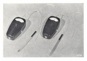
Fig. 1. Left, the electrical clinical thermometer, consisting of a probe and an indicating instrument, connected by a flex. The button visible on the right of the instrument is pressed in order to take a reading. The reading may be taken about 13 seconds after insertion of the probe. Right, the model for skin thermometry.
