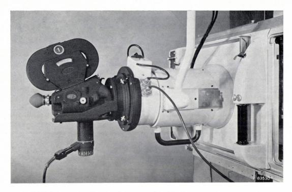
Fig. 1. Apparatus for cinematography with the image intensifier. Right: Viewing system on the stand of an ordinary diagnostic X-ray installation. The usual fluorescent screen is replaced by an image intensifier. Left: The film camera, with the film magazine on top; an eyepiece to view the image during the taking of the film is at extreme left, on the axis of the camera and image intensifier (see III).
