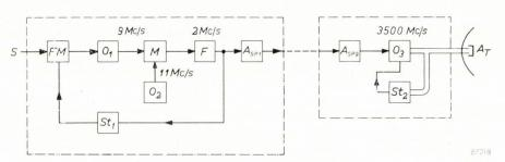
Fig. 8. Block diagram of the transmitter of fig. 7. The left-hand part, surrounded by the dotted line, is built into the rack; the right-hand part, is built into the reflector assembly.
