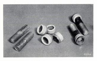
Fig. 5. Threaded studs  $({}^{1}/_{2}\text{-inch})$  and the corresponding welding cartridges. Two studs with cartridges fitted are shown on the right of the picture.
