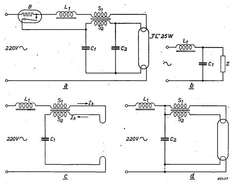
Fig. 1. a) Circuit diagram of a ballast for "TL" 25 W lamp, which was on the market in 1945.  $L_1$  choke coil and  $C_1$  capacitor slightly off resonance with the supply frequency.  $S_1/S_2$  double choke.  $C_2$  capacitor for interference suppression. B bimetal relay (excess current safety device).
