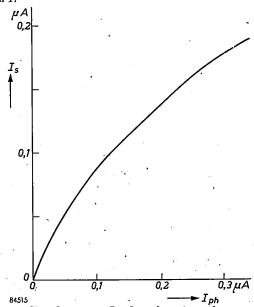
Fig. 4. Signal current  $I_s$  plotted against photo-current  $I_{\rm ph}$  for image iconoscope 5854.
