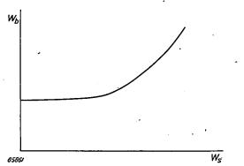
Fig. 11. Noise power  $W_b$  in one of the channels, plotted as a function of the power  $W_s$  supplied to the other channels. The curve applies to one specific ratio between the level of the signal to be transmitted and the frequency swing.
