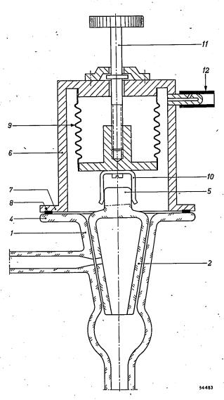
Fig. 2. New high-vacuum tap with short outgassing time. I tap housing with glass flange 4. 2 plug with square, solid head 5. 6 metal cap, with flange 7, carrying sealing ring 8. 9 metal bellows. 10 sprung fork. 11 adjusting screw. 12 valve. After the tap is outgassed, the cap is removed.
