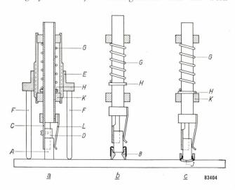
Fig. 6. Diagram to demonstrate the operation of the welding gun.
