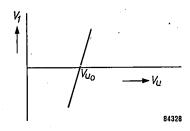
Fig. 8. Relationship between  $V_{\rm u}$  and  $V_{\rm 1}$  (fig. 7).  $V_{\rm 1}$  is a measure of the deviation of  $V_{\rm u}$  from its nominal value  $V_{\rm u_0}$ .
