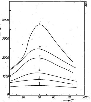
Fig. 6.  $\varepsilon$ -T curves for sintered specimens, composed of BaTiO<sub>3</sub>, SrTiO<sub>3</sub> and CaTiO<sub>3</sub>, corresponding to the compositions I to  $\delta$  in fig. 5. Compositions 3 to  $\delta$  lie in the two-phase region and in this order contain increasing amounts of the phase rich in CaTiO<sub>3</sub>, which makes the  $\varepsilon$ -T curves increasingly flat.
