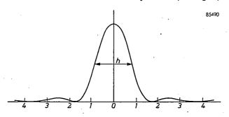
Fig. 5. Schematic directional diagram of a parabolic antenna. The ordinate represents the relative sensitivity, whilst the abscissa represents the direction relative to the axis, plotted in arbitrary units of angular measure. h is the half width of the "major lobe".
