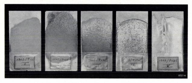
Fig. 6. Photographs of glaze samples, heated to points I-V indicated in fig. 5.
