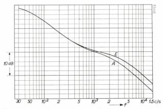
Fig. 3. Proposals for a standard reproduction channel for long-playing records, submitted to the I.E.C. for consideration. The speed v of the needle point for a constant sound intensity is plotted along the vertical axis. Along the horizontal axis the frequency f is plotted. Both are on a logarithmic scale. Curve A corresponds to the American proposal, curve E to the European proposal.
