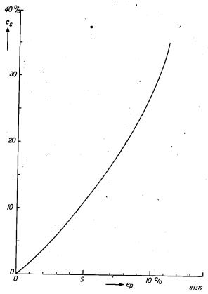
Fig. 2. Relationship between the relative voltage losses  $e_s$  and  $e_p$ , in a series and a parallel system respectively, the copper volume, mains voltage, and overall runway lighting power being the same in both cases.
