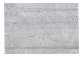
Fig. 10. As fig. 9, but recorded during the welding of a  $\frac{1}{2}$ -inch stud with a coarse thread on the end to be welded. The stud then drops intermittently, thus producing an inferior weld. Premature melting of the screw thread is a possible cause.
