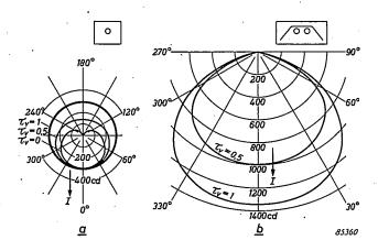
Fig. 2. a) Light distribution curves for normal "TL" lamps coated on the upper surface with a uniform layer of dirt, having a transmission factor  $\tau_{\rm v}$ . The curve for  $\tau_{\rm v}=1$  (clean lamp) is identical to that in fig. 1a.
