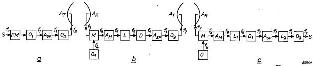
Fig. 5. Block diagram of a transmitter (a), a relay station (b), and a terminal station (c), using an oscillating transmitting tube and a system of double modulation.
