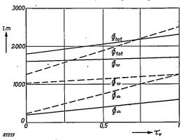
Fig. 9. Effect of a dirt layer on the upper surface on the performance of "TL"F lamps (full lines) and of normal "TL" lamps (dotted lines). The transmission factor  $\tau_{\rm v}$  of a uniform layer of dirt on the upper surface is plotted horizontally, whilst the total luminous flux  $\Phi_{\rm tot}$ , and the luminous flux radiated into the lower and upper hemispheres,  $\Phi_{\rm D}$  and  $\Phi_{\rm D}$  respectively, are plotted vertically.
