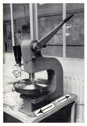
Fig. 10. Centring a matrix. The latter is loosely champed to a rotatable table. The position is altered until on turning the table, the grooves, viewed through a microscope, are seen to move in one direction only (either inwards or outwards). The lever is then pulled down, punching out the centre hole.
