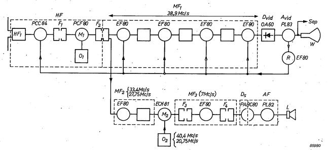
Fig. 7. Block diagram of the television receiver for four standards. HF high frequency section (incorporating the channel selector, see fig. 3), with high frequency stage  $HF_1$ , high-frequency band filter  $F_1$ , first oscillator  $O_1$ , first frequency changer  $M_1$  and part of the I.F. band filter  $F_2$ . Vision channel: MF1 intermediate frequency amplifier with
