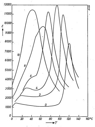
Fig. 3.  $\varepsilon$ -T curves for mixed crystals of BaTiO<sub>3</sub> and BaSnO<sub>3</sub>. The figures beside the lines give the percentage of BaSnO<sub>3</sub> present. The mixed crystals have a higher  $\varepsilon$  maximum than pure BaTiO<sub>3</sub>. For specimens where the first and second maxima lie close together (see fig. 4) a disturbance occurs which makes this effect less obvious.
