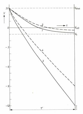
Fig. 8. 1 and 2 are  $V=\mathbf{f}(t)$  curves, as shown in fig. 3b, for the image iconoscope. 3 and 4 refer to the "Scenioscope" (slightly conductive target, signal plate potential negative), 3 for a non-illuminated, and 4 for a faintly illuminated photo-cathode.
