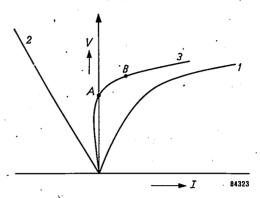
Fig. 2. Relationship between current and voltage for 1) choke (as in fig. 1); 2) condenser; 3) choke and condenser in parallel.
