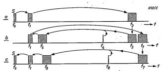
Fig. 6: Schematic representation of the frequencies of the signal voltages in a transmitter (a), a relay station (b), and a terminal station (c), for a circuit according to fig. 5.
