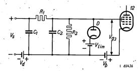
Fig. 5. Circuit of the delay network 11 of fig. 4. Vs input signal (varying direct voltage). Vd threshold voltage. C1 capactitor from which capacitor  $C_2$  is given a delayed charge via resistor  $R_1$ .  $R_2$  discharge resistor. The diode D with bias  $V_{\text{lim}}$  forms the limiter. Vb grid bias. 12 reactance tube.
