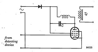
Fig. 14. Amplifier of the "Balham" stabilizer. A pulsating direct voltage is applied to anode and screen grid of the tube, so that this tube functions as a rectifier; the current through the D.C. winding of transductor Td in the anode circuit is dependent on the alternating voltage on the grid.
