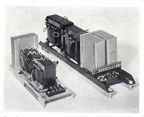
Fig. 6. Two magnetic stabilizers on the principle of fig. 4, one having an output of  $80~\mathrm{VA}$  and the other of  $300~\mathrm{VA}$ .
