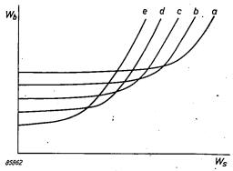
Fig. 12. Noise power  $W_b$  in one of the channels, plotted as a function of the power  $W_s$  supplied to the other channels, for various values of the frequency swing. For a given signal level, the frequency swing increases from a to e.
