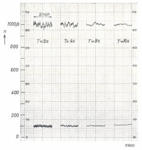
Fig. 8. The "jitter" of the recorded trace, which is due to the statistical fluctuations of the counting rate, diminishes with increasing time constant T. The recordings shown were made at a fixed position of the detector, with counting rates  $n=1000/\mathrm{sec}$  and  $n=100/\mathrm{sec}$ .
