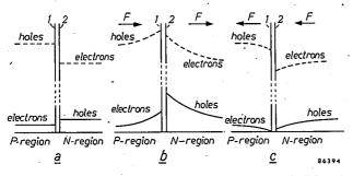
Fig. 1. Concentrations of minority charge carriers (full lines) and of majority charge carriers (broken lines), as functions of position on either side of a P-Njunction in a germanium crystal. The concentration of majority charge carriers in practice is between  $10^4$  and  $10^6$  times that of the minority charge carriers. 1 and 2 denote the boundary planes of the junction.
