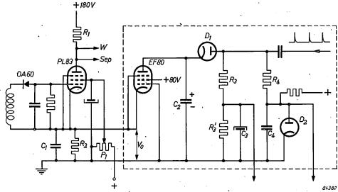
Fig. 8. Diagram of the video stage. Video detector is the germanium diode OA 60, video amplifier the pentode PL 83. The signal at the anode of the PL 83 controls the picture tube (W) and the separator (Sep), which separates out the synchronizing signals.  $P_1$  contrast control.
