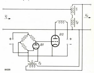
Fig. 10. Simplified circuit diagram of the equipments of fig. 9. The bridge incorporating the diode  $B_1$  becomes unbalanced if the filament voltage of  $B_1$  deviates from its nominal value; the bridge thus acts as detecting device.
