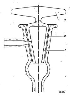
Fig. 1. Glass high-vacuum tap of normal construction.  ${\it I}$  tap housing.  ${\it 2}$  plug.  ${\it 3}$  handle.
