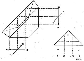
Fig. 7. Roof prism. The 45° prism inverts the image, that is, changes direction B-O; it is seen from the bottom right-hand diagram that a roof prism (two reflecting planes making an angle of 90°) also reverses the image laterally so that L and R are exchanged.
