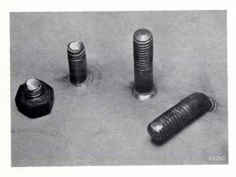
Fig. 13. Simple tests to determine the mechanical strength of the joint between stud and work. Right: a stud bent through 90° by hammering. Left: a stud sheared off by turning a nut against a metal sleeve (not shown in the photograph) fitted round the stud. The part of the stud broken off, with the nut still on it, is seen on the extreme left of the picture.
