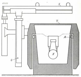
Fig. 5. Cross-section of the "Symmetrix" table. The base forms a U, over which the table, with its two sidewalls, fits as an inverted U. G is the mounting of the viewing system S. For the other letters see fig. 1 and fig. 3.
