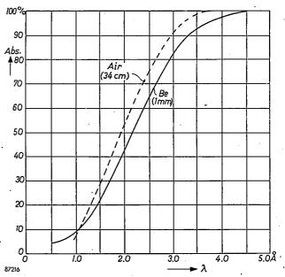
Fig. 11. The percentage absorption of a 1 mm thick beryllium window and of an air path 34 cm long (i.e. about the length used in the "Norelco" spectrograph) as a function of wavelength  $\lambda$  of the X-rays.
