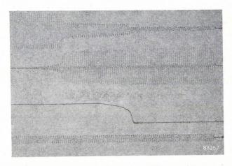
Fig. 9. Diagram recorded during the welding of a ½-inch stud. Starting at the top we have, plotted against time: the voltage, the current, the displacement of the stud, and a constant 50 c/s A.C. voltage which serves as a time scale.
