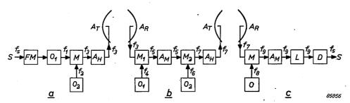
Fig. 1. Block diagrams of a transmitter (a), a relay station (b), and a terminal station (c), using an amplifying tube in transmitter and relay station. The significance of the letters is given in the text.
