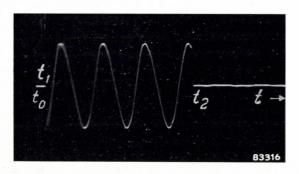
Fig. 8. Oscillogram referring to fig. 7. At  $t=t_0$ , the push button of  $S_2$  is pressed, with  $S_1$  already closed. After a certain delay, depending upon the design of  $S_1$ , the contacts of  $S_1$  open, that is at  $t=t_1$ . A 50 c/s voltage then appears on the oscilloscope; this voltage is suppressed when  $S_2$  closes (at  $t=t_2$ ). The interval between  $t_1$  and  $t_2$  is  $3\frac{1}{2}$  cycles.
