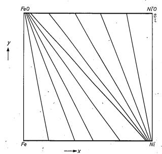
Fig. 9. Phase diagram for the system Fe-Ni-FeO-NiO (schematic). This diagram serves to elucidate fig. 7. The connodes have been drawn in order to demonstrate that the combination Ni + FeO is more stable than the combination Fe + NiO.
