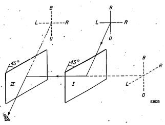
Fig. 4. The reflection at mirror I produces a virtual image in the form of "mirror writing"; it is re-converted to legible writing by reflection at mirror II.
