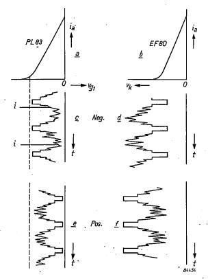
Fig. 11. a) Anode current  $i_a$  as a function of the control grid voltage  $v_{g1}$ , for the video tube PL 83. b)  $i_a$  as function of the cathode voltage  $v_k$  (with earthed grid), for the control tube EF 80. c) Control grid voltage of the PL 83, and d) cathode voltage of the EF 80 as a function of the time t, with negative picture-modulation; e) and f) the same for positive picture-modulation.
