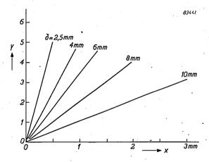
Fig. 8. The voltage y (fig. 7) plotted on an arbitrary scale as a function of the deflection x of the armature from the central position for various values of the air gap  $\delta$ .
