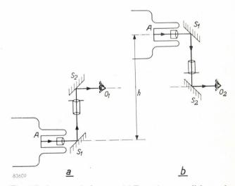
Fig. 6. Periscope optical system. (a) Two mirrors parallel to each other  $(S_1 \text{ and } S_2)$  bend the path of rays, but do not change the position of the observed image. (b) By rotating the whole system about axis  $AS_1$ , the image intensifier can be raised or lowered a distance h without varying the level of the eye  $(O_1 \text{ or } O_2)$ . The direction of observation can be varied by tilting mirror  $S_2$  about an axis perpendicular to the plane of the drawing.
