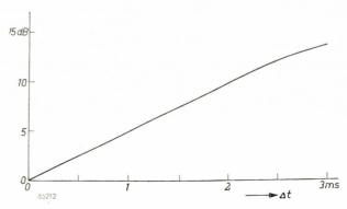
Fig. 10. Differences in intensity (in dB) plotted against the phase differences  $\Delta t$  which produce the same angular displacement of the sound image.
