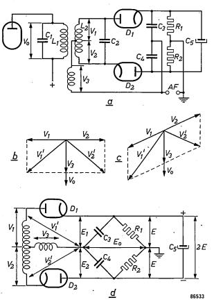
Fig. 4. a) Circuit of ratio detector.  $L_1$ - $C_1$ - $L_2$ - $C_2$  last I.F. bandpass filter. AF terminals across which the audio frequency voltage appears.
