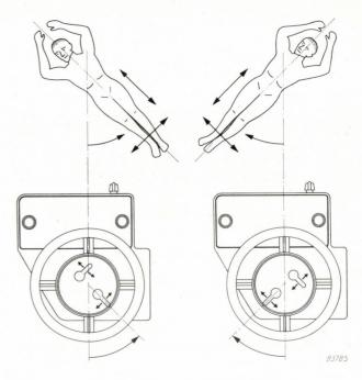
Fig. 8. The hub of the hand wheel driven by a small motor housed in the control box, rotates with the patient so as to maintain the switches in the same positions relative to the patient-movements controlled by them.
