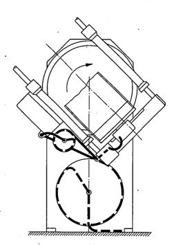
Fig. 6. Connecting cables on the equipment. During all movements, cable sections a and b are held taut between terminal points I, II and III by spring-loaded cable-drums A and B. Section c is prevented from sagging by a wire spiral fitted round it. Other components numbered as in fig. 5. The diagram on the right shows the change in the configuration of the cable sections when the patient is adjusted to another position.
