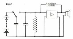
Fig. 2. Circuit diagram of the electronic bass drum.
