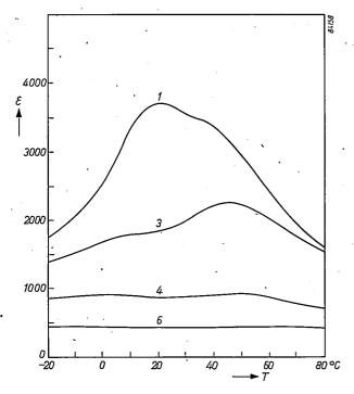
Fig. 11.  $\varepsilon$ -T curves for a series of specimens in the BaTiO<sub>3</sub>-SrTiO<sub>3</sub>-CaTiO<sub>3</sub> system to which about 10% Mg<sub>2</sub>TiO<sub>4</sub> has been added. The compositions (calculated without the Mg<sub>2</sub>TiO<sub>4</sub>) of 1,3,4 and 6 correspond approximately with the similarly numbered points in fig. 5. The effect of the additive is to make the curves flatter than those in fig. 6.
