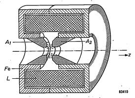
Fig. 2. Magnetic electron lens. L coil, Fe iron jacket,  $A_1$ ,  $A_2$  pole pieces. The electrons move close to the z-axis, which is the axis of rotational symmetry of the magnetic field of the lens.
