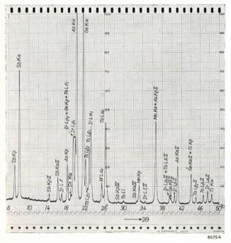
Fig. 6. Qualitative analysis of a mixture of several elements using a quartz analyzing crystal ( $10\overline{11}$ -plane), scintillation counter, scanning speed  $^{1}/_{2}{}^{\circ}$  per minute. The K-spectra of 22 Ti, 25 Mn, 32 Ge, 33 As, 34 Se, 51 Sb and the L-spectra of 73 Ta, 74 W and 77 Ir can be seen. (The higher order reflections are indicated by Roman numerals.)
