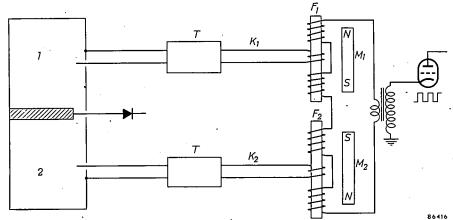
Fig. 5. Diagram of modulation system. The coaxial lines  $K_1$  and  $K_2$  couple the resonators I and I to the ferroxcube rods I and I, which are successively magnetized by an alternating current of rectangular waveform. The permanent magnets I and I pre-magnetize the ferroxcube in opposite directions; I matching transformers.
