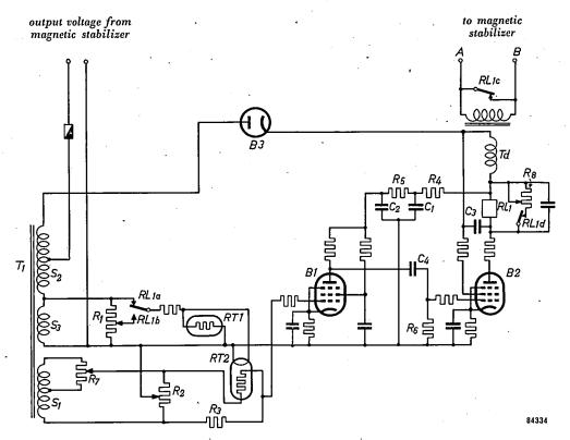
Fig. 15. Circuit diagram of the "Balham" stabilizer. The "magnetic" part is not shown. The A.C. coil of the transductor is assumed to be connected between the points A and B of fig. 4 or fig. 5.
