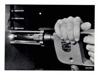
Fig. 7. Welding a  $^3/_8$ -inch stud to a vertical wall by the new method with a welding cartridge.
