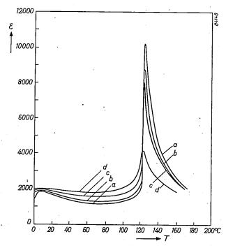
Fig. 1. The dielectric constant  $\varepsilon$  of BaTiO<sub>3</sub> as a function of temperature T. The curves a, b, c, d have been measured for specimens sintered at 1400, 1350, 1300 and 1280 °C respectively. In the same order the size of the crystals decreases from about 100  $\mu$  to 5  $\mu$ . The maximum at 123 °C corresponds to the transition from cubic to tetragonal structure, the maximum at about 10 °C to the transition from the tetragonal to the rhombic structure.
