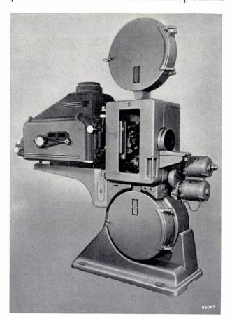
Fig. 4. The 70 mm film projector (type EL 4000) which at the same time is suitable for projecting normal 35 mm and "CinemaScope" films (with 4 magnetic sound-tracks or with one optical sound-track).
