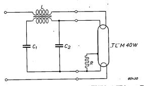
Fig. 4. Circuit diagram of ballast for "TL"M 40 W lamp. The two coils L on one core possess a certain leakage.  $C_1$  resonance capacitor. C2 capacitor for interference suppression. R resistor of 1 MΩ connecting the conductive strip to one of the electrodes.
