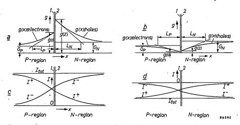
Fig. 3. Variation of the concentration g of the minority charge carriers (electrons in the P-region and holes in the N-region) at the P-N junction. The concentration gradients occurring at the boundary planes 1 and 2 of the junction can be read off the figure, after which the minority currents themselves can be written down directly.  $L_P$  and  $L_N$  are the diffusion lengths in the P and N regions respectively.
